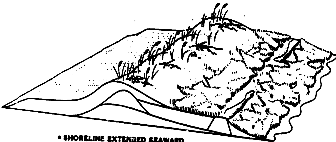
Figure 14. PHASE II COMPLETED SHORELINE AND BARRIER ISLAND NOURISHED
